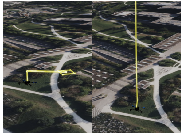
Fig. 6. Comparison of expected mission flight path (left) with rapidly ascending flight behavior (right) caused by pairwise misconfigurations.
